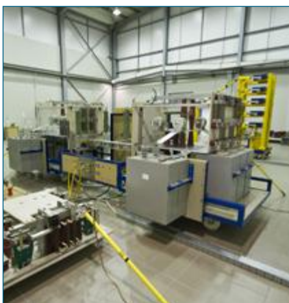
100kA, 10/350µsec. Impulse current generator (1)
