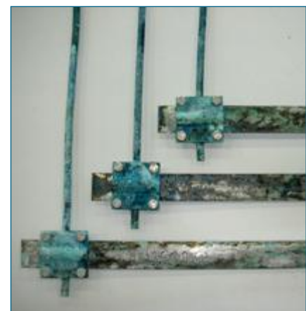
Overview of samples after the humid sulphurous atmosphere testing
